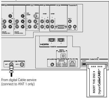
This cable should be connected to ANT 1 terminal directly. If you connect the cable via a VCR, the TV may not receive the signals correctly.
